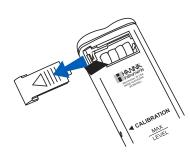
DiST® is provided with Battery Error Prevention System (BEPS), which avoids any erroneous reading due to low battery level, by switching the meter off. To change the batteries, slide off the battery compartment cover and replace all four 1.5 V batteries while paying attention to their polarity.
